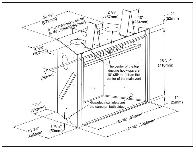
Figure 1. Dimensions of the Firebox.
